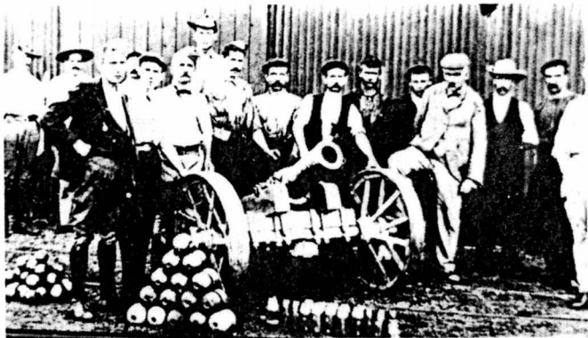
The artillery piece which was made in Mafeking. This was a 4½" Howitzer and the barrel was made by shrinking rings of iron upon an old iron drain pipe. The result was a smooth bore gun which according to the literature was found most serviceable.
